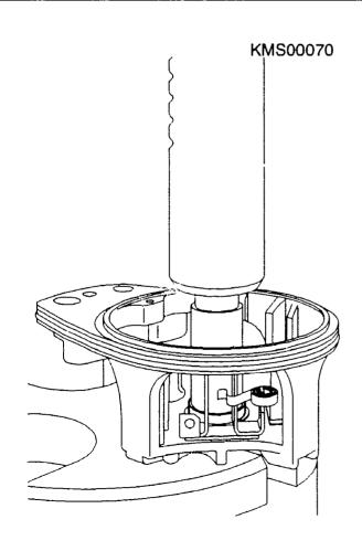
CHECKING AND REPAIRING COMPONENTS Checking commutator end shield Check all carbon-brush holders insulated against commutator end shield for ground short. ("+" carbon-brush holders/insulated "-" carbon-brush holders) Interturn short-circuit tester 0 986 619 110 Test prods 0 986 619 114 Ground-short test voltage: 80 V
